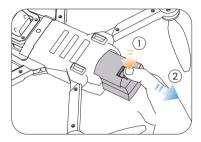
Press the lock button on the battery, and pull the battery out from the drone.
