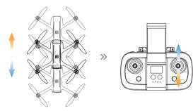
3 Deactivate Trim Mode: Once adjustments are made, long press the Trim buttor or stop operating the joysticks for 2 seconds to exit Trim Mode.
