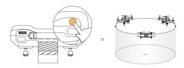
Long press the 5 button, the drone will enter the Circle Fly mode. Exit the Circle Fly mode by long pressing the same button again or pushing the right joystick in any direction.
