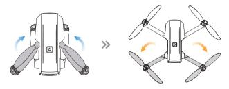
All arms of the drone are folded before the drone is packaged at the factory. First, unfold the front arms, then unfold the rear arms
