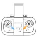
Simultaneously push the left joystick to the bottom right corner and the right joystick to the bottom left corner. The motors will rotate, and the drone is unlocked.
