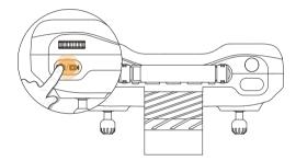
**Take Photo:** Short press the button on the transmitter to take a photo. The transmitter will beep once, signaling that a photo has been taken.
