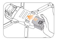
Push the battery correctly into the drone. Make sure that you hear a click sound, which indicates that the battery is firmly installed.
