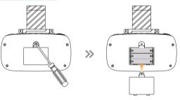
Open the battery cover on the back of the transmitter. Put in three AAA batteries (not included). Then, close the cover.
