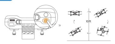
After you get familiar with all the functions of the drone, you can try this amazing flip mode. When the drone is at least 10 ft from the ground, press down on the button, then push the right joystick in any direction. The drone will perform a flip toward that direction
