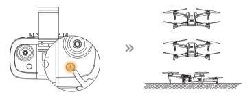
1 The Emergency Stop function should only be used in an emergency during the flight to avoid any damage or injury. Long Press the button. The transmitter will long beep once. The drone will fall down immediately.
