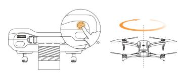
Short press the 🥳 button, the drone will enter the High Speed Rotation mode. Exit the High Speed Rotation mode by pressing the same button again or pushing the right joystick in any direction.
