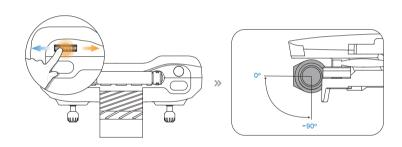
Adjust the camera angle by scrolling the camera adjustment dial (tilt range: -90°~0°)
